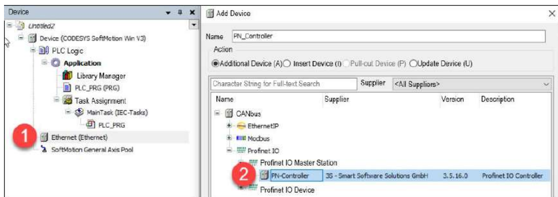
Figure 5-2-36 Adding PROFINET IO master station
