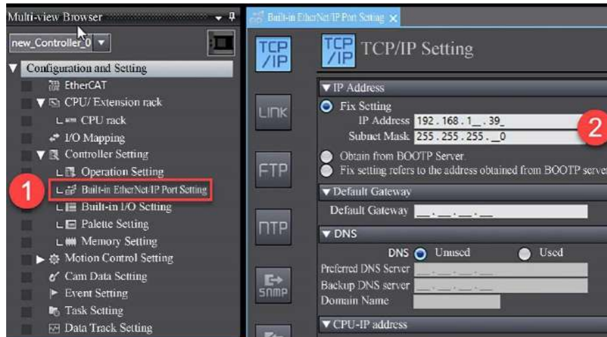
Figure 5-7-25 EtherNet/IP port Settings
