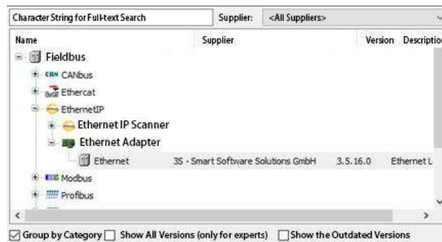
Figure 5-7-14 Adding an Ethernet adapter
