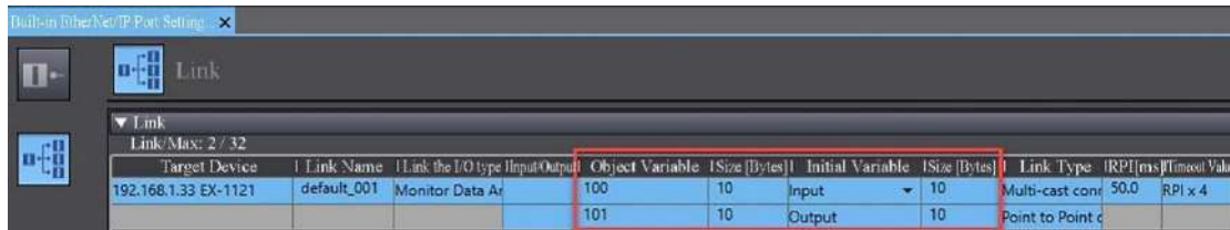
Figure 5-8-33 Setting target device parameters
