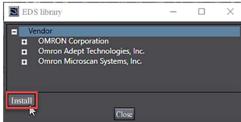
Figure 5-7-30 Installing the EDS file
