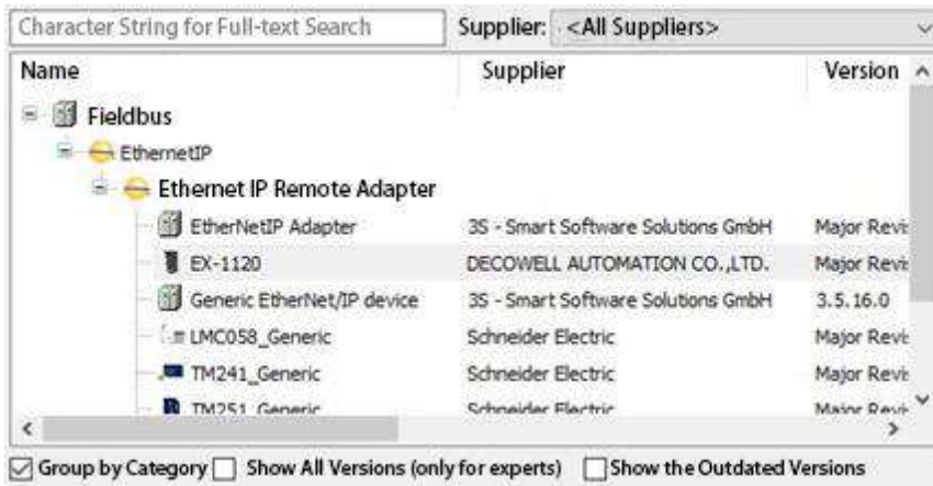
Figure 5-7-17 Adding the EX-1120 adapter
