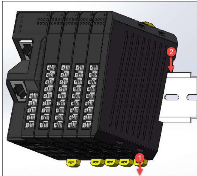
Figure 3-2 Installing an entire module group
