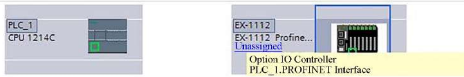
Figure 5-9-6 Assigning IO controllers
